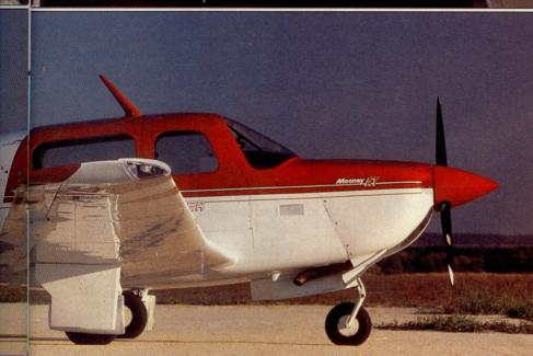
ram air inlet, a small portal beneath the spinner that, when opened at altitude, increases manifold pressure about one inch by by-passing the air filter. The AT will be flown at relatively low altitudes most of the time, so the ram air feature isn't needed. In addition to saving a few dollars in materials and manufacturing costs, eliminating the ram air precludes the possibility of a student opening the inlet on the ground and the engine ingesting harmful dust and dirt.
